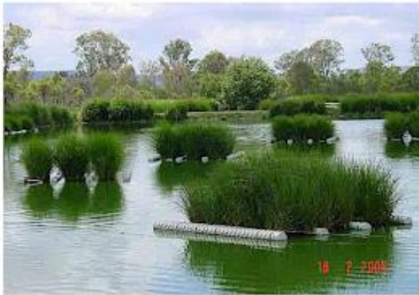
Pantoons in an effluent pond at Toogoolawah
